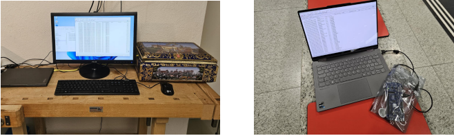
Fig. 2: Data Acquisition Setups; (left) isolated basement with Faraday cage, (right) open view train station bench
