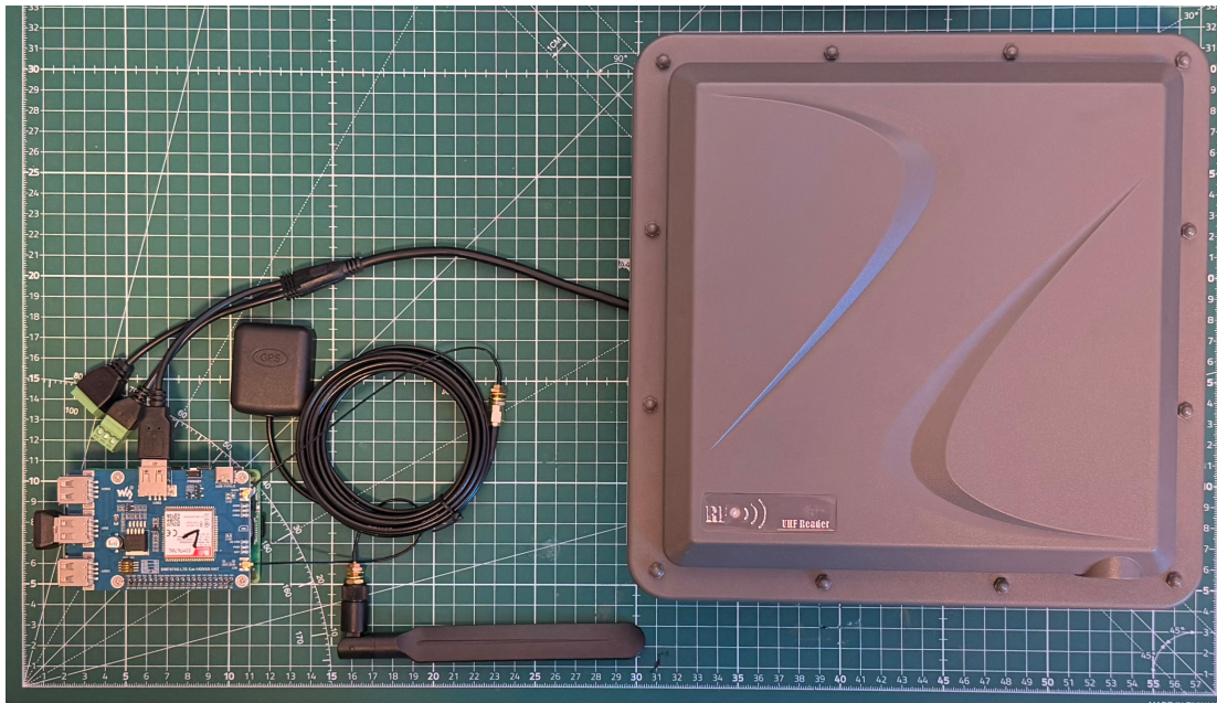
Figure 4.3: Truck-side tracker prototype with Raspberry Pi 5, the SIM7670G LTE/GNSS HAT, the RFID reader antenna, the GNSS antenna, and the LTE antenna attached.
