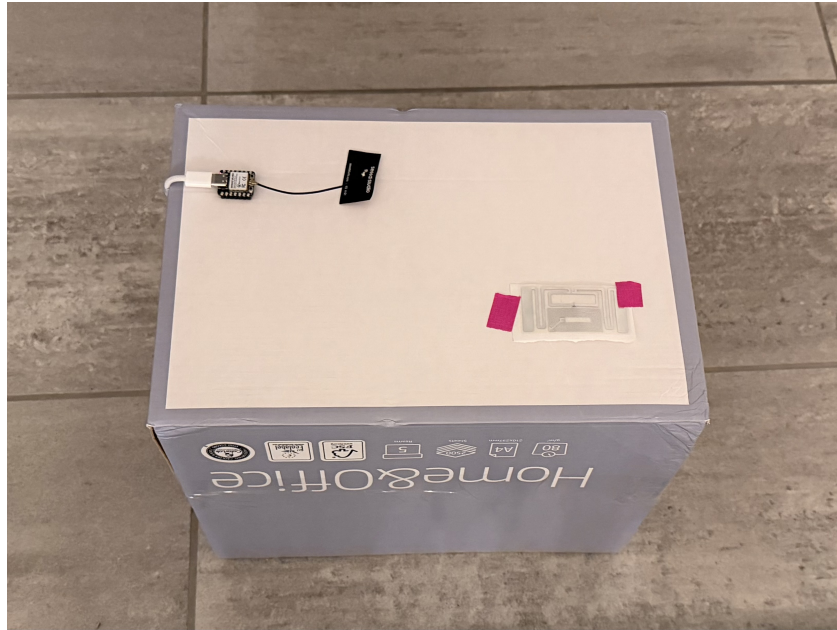
Figure 5.4: Box-mounted BLE beacon and RFID tag used in the simulated 18 t rigid-truck layout.
