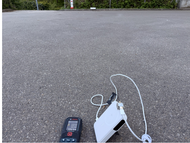
Figure 5.2: Outdoor BLE range-test setup with the BLE beacon connected to a battery pack and the distance meter in the foreground, and the pi-5-gateway-01 on top of a cardboard box visible in the distance.
