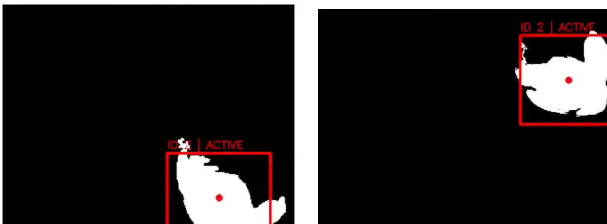
Figure 4.7: Kalman tracker estimating the changing position of a moving agent across time.
