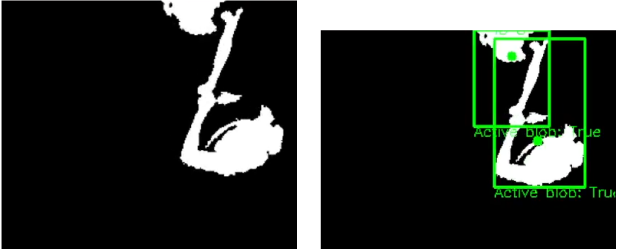
Figure 4.5: Superblob splitting during a handshake using depth local-maxima extraction and Watershed. Left: foreground mask showing a continuous superblob. Right: individual sub-blobs recovered for each agent.
