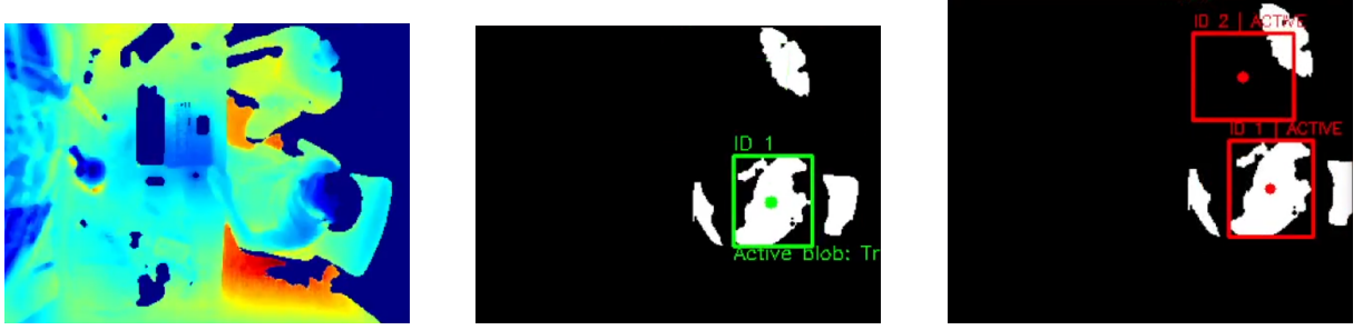
(a) Missed blob in the foreground mask. The Kalman filter continues estimating from the motion model.
