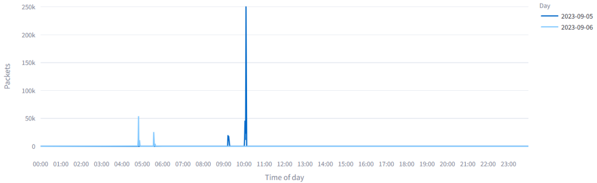
Figure 6.4: Web browsing packets per minute over the day for two adjacent dates. Narrow spikes indicate short-lived activity windows (could indicate downloads or update checks).
